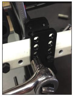
**Step 4:** Place the universal caliper brackets outside the OEM axle brackets and loosely install the 5/16" x 2.25 bolts supplied.
