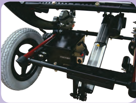
Tilt Actuator And Battery Box
